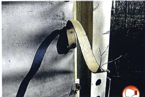
Tarpaulin strap Damaged strap (rear right side)
