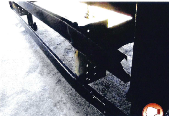
Sideguards Deformed sideguards
