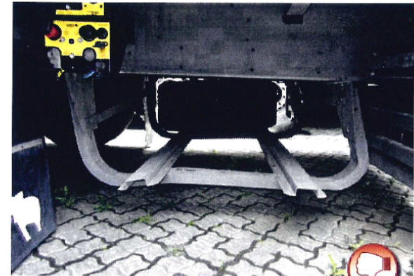
Spare wheel holder Deformed spare wheel holder
